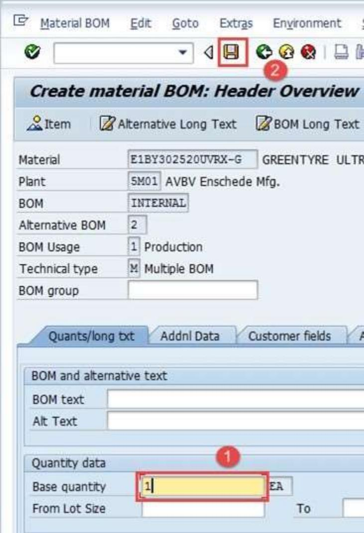
The screenshot shows the SAP 'Create material BOM: Header Overview' screen. The toolbar at the top contains a 'Save' icon (floppy disk) which is highlighted with a red box and a red circle containing the number '2'. Below the toolbar, the 'Create material BOM: Header Overview' section contains the following fields:
